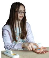
The **Biox Epsilon** E100 is a contact imaging system with a linear and calibrated response for characterising near-surface properties of skin and other electrically insulating materials. You can use it, for example, to measure stratum corneum hydration and imperceptible perspiration even with poor skin (hair, wrinkles, etc). For more information, see [www.biox.biz](http://www.biox.biz).
